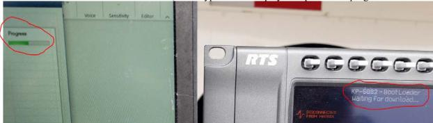
Once the upload is complete, power cycle the keypanel to verify the new connection scheme is activated. RVON or OMENO depending on which firmware was uploaded.
