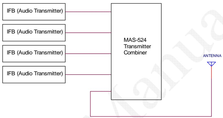
This application features no additional amplification. Used when the coverage area is a small stage or similar which does not require full, legal limit RF energy.
