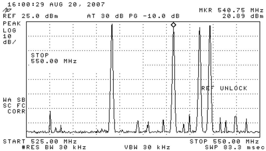
Spectrum analyzer display showing the four carriers after optimization.
