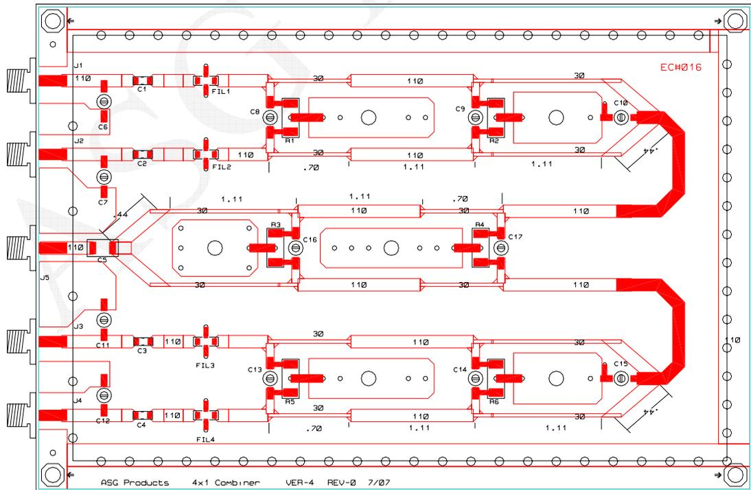
Interior of the combiner PCB showing locations of the adjustment capacitors.
