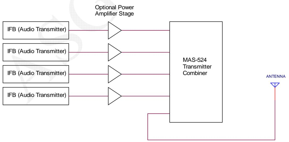
This application uses additional amplification. Ideal for large areas or for splitting the output to multiple transmit antennas for coverage in complex facilities with multiple stages. Proper amplification can yield full legal limit energy on each carrier on multiple antennas.
