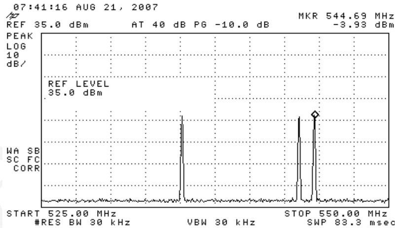
**Adjacent channel leakage. (Input #1,3,4 Driven with +30dBm; Input #2 Analyzed)**
